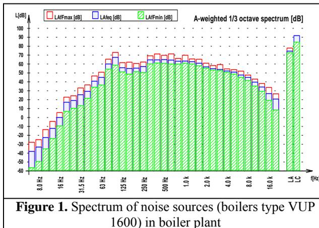
**Figure 1.** Spectrum of noise sources (boilers type VUP 1600) in boiler plant
