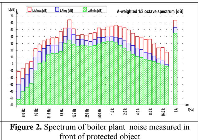
**Figure 2.** Spectrum of boiler plant noise measured in front of protected object
