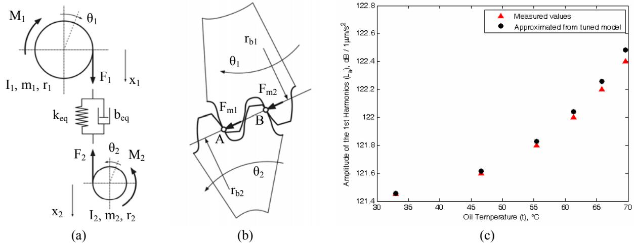
**Figure 2.** (a) 2DOF model of meshing gears; (b) action line and forces applied in meshing points (after [5]); (c) Amplitude of 1<sup>st</sup> tooth meshing harmonics as a function of oil temperature.
